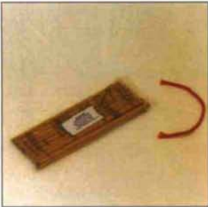
Figure 8 Portfire (left) and slow-burning wick (right), used to light fireworks
